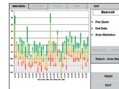
Area Analysis Display Displays maximum average and minimum values of frequencies within the specified region.
